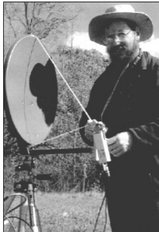
Fig 17.43: Using a knot tied in a piece of string to accurately place the feed horn at the focus of an offset dish
