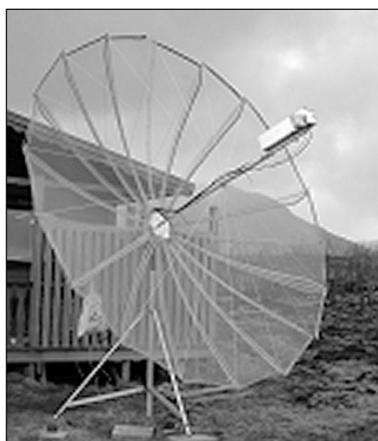
Fig 17.45: Parabolic preloaded stressed dish for moonbounce used by Michael Kohla, DL1YMK, in Iceland
