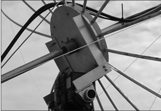
Fig 17.46: Bush arrangement at the centre of the dish
