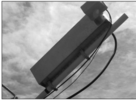
Fig 17.49: Square waveguide feeder built by Zdenek Samek, OK1DFC, fitted to the pre-loaded stressed dish
